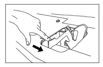
Then go to the front of the vehicle and push the secondary hood release handle toward the driver side of the vehicle.
